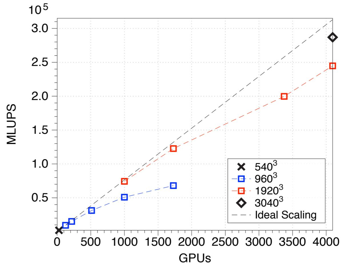
*Parallel performance in million-lattice updates per second (MLUPS) for multiphase lattice Boltzmann simulator on Titan (90% parallel efficiency on 4,096 compute nodes)*
