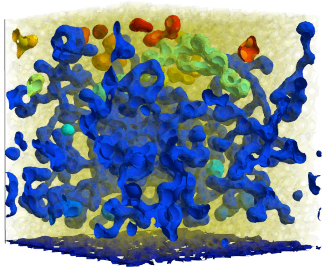
*Connected components analysis applied to identify connected portions of a phase within simulation*
