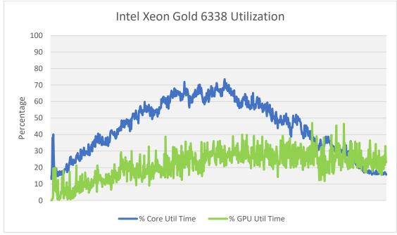
The following graph illustrates CPU Core utilization using an Intel Xeon Gold 6338 3.2 GHz Turbo (Skylake) for 64 VMs. This server configuration has 64 cores with hyperthreading enabled.
