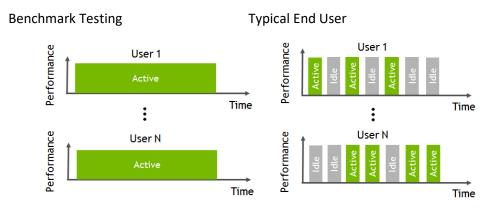
NVIDIA used the nVector benchmarking engine to conduct vGPU testing at scale. This benchmarking engine automates the testing process from provisioning virtual machines, establishing remote connections, executing KW workflow, and analyzing the results across all virtual machines. Test
