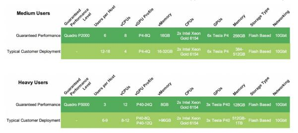
NVIDIA recommends configuring your dual socket server of choice using the Intel Xeon Gold 6154 CPU. The high frequency of 3.0 GHz alongside 18 cores of the CPU are well suited for optimal performance for each end user while supporting the highest user scale on the server which makes it also a cost-effective solution for Siemens NX.
