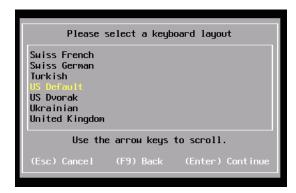
Select your desired keyboard layout using the arrow keys and then press [ENTER]. The Enter a root password window displays.
