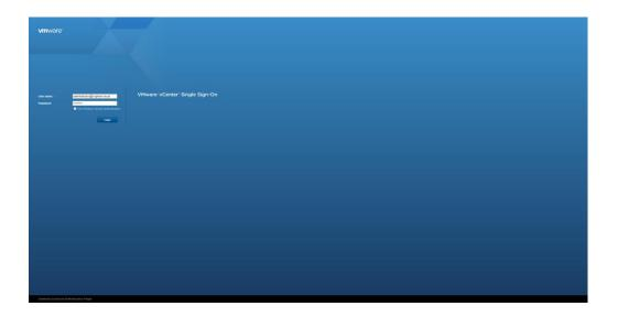
**2.** Enter the username and password that you specified during installation, and then click the **Login** button. The *VMware vSphere Web Client* page displays.
