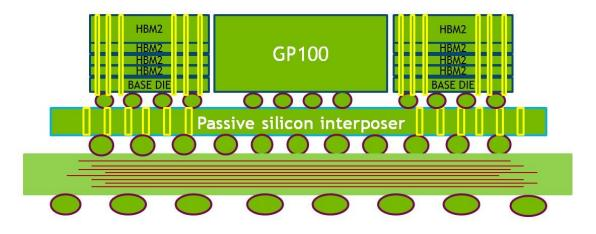
Figure 9. Cross-section Illustrating GP100 adjacent HBM2 stacks
