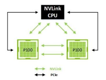
Figure 17. Two GPUs and a CPU Connected with 80 GB/sec Bidirectional Bandwidth NVLink Interfaces
