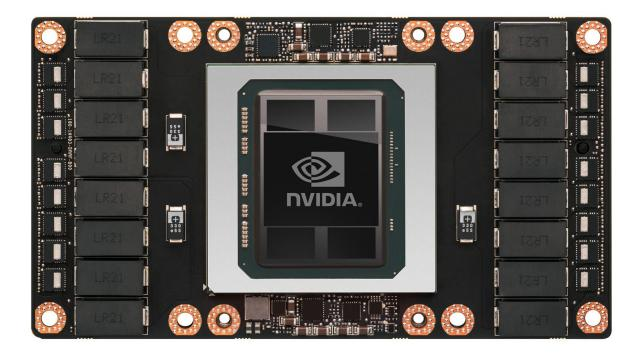
Figure 11. Tesla P100 Accelerator (Front)
