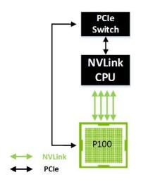
Figure 16. NVLink GPU-to-CPU Interconnect
