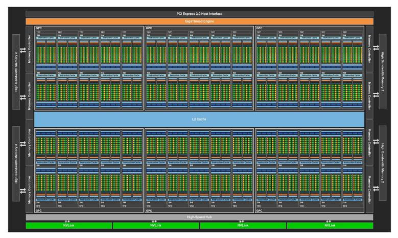
Figure 7. Pascal GP100 Full GPU with 60 SM Units
