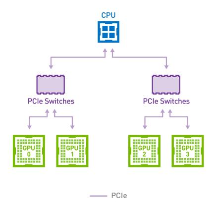
*Figure 11* A common PCIe topology for 4 GPUs attached to a single CPU. Purple arrows represent PCIe x16 connections
