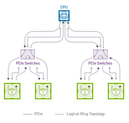
Figure 12 Ring order of GPUs in PCIe tree
