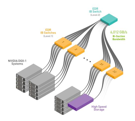
Figure 8 Example Multi-System Cluster of 124 DGX-1 Systems Tuned for Deep Learning
