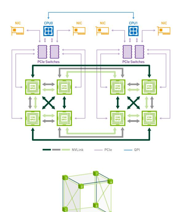
*Figure 4* DGX-1 uses an 8-GPU hybrid cube-mesh interconnection network topology. The corners of the mesh-connected faces of the cube are connected to the PCIe tree network, which also connects to the CPUs and NICs.
