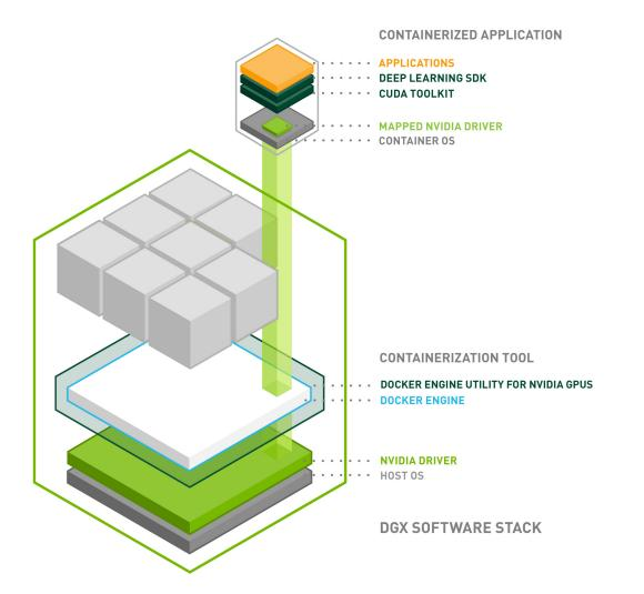
*Figure 10* Docker containers encapsulate application dependencies to provide reproducible and reliable execution. The Docker Engine Utility for NVIDIA GPUs maps the user-mode components of the NVIDIA driver and the GPUs into the Docker container at launch.
