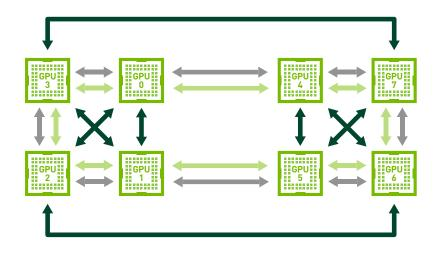
*Figure 13* The DGX-1 NVLink hybrid cube-mesh topology can be treated as three interwoven bidirectional rings of single NVLink connections, shown here in gray, light green, and dark green.
