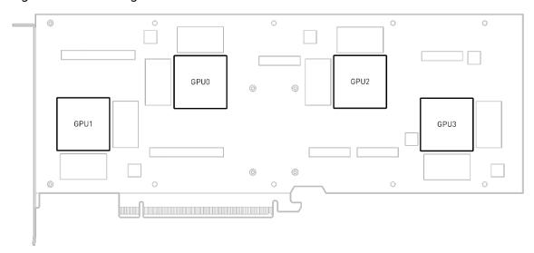
Figure 1. Single Board with Four GPUs
