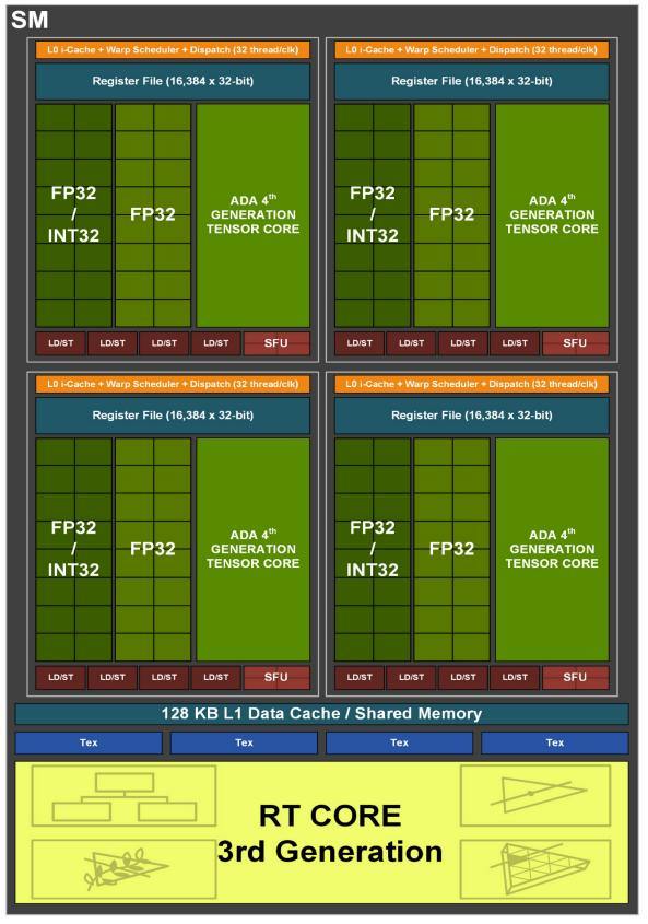
Figure 5. Ada Streaming Multiprocessor (SM)
