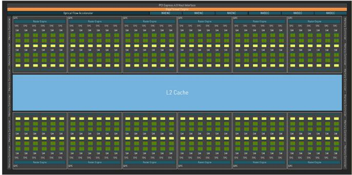
**Note:** The AD102 GPU also includes 288 FP64 Cores (2 per SM) which are not depicted in the above diagram. The FP64 TFLOP rate is 1/64th the TFLOP rate of FP32 operations. The small number of FP64 Cores are included to ensure any programs with FP64 code operate correctly, including FP64 Tensor Core code.
