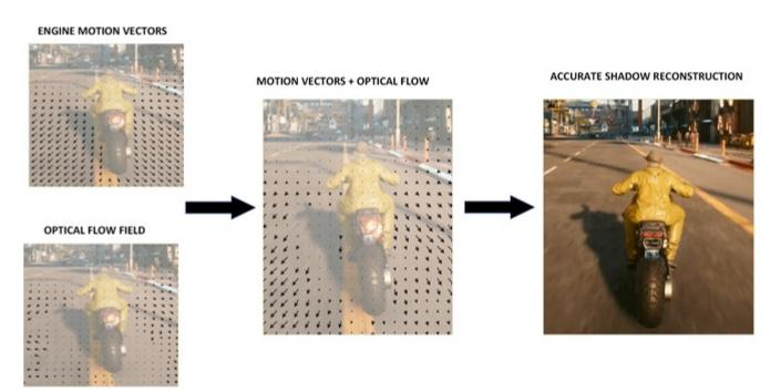
To generate more accurate frames without distracting artifacts, DLSS 3 combines 3D engine motion vectors with the OFA Engine's optical flow field.
