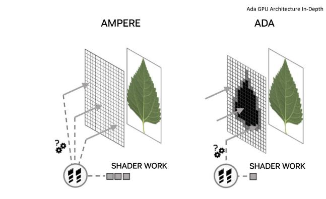
Ada's Opacity Micromap Engine with opacity mask reduces shader work compared to Ampere
