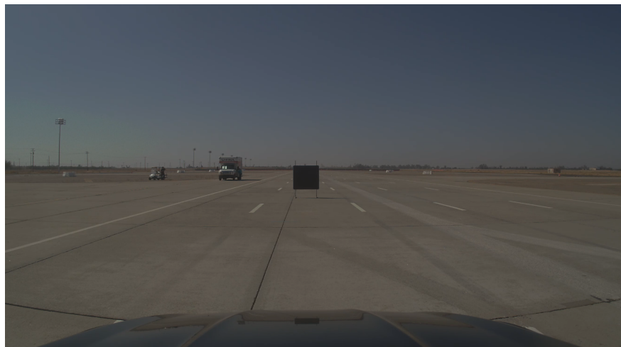
Figure 13: Reflective panel with 5% reflectiveness at 20m away from ego vehicle
