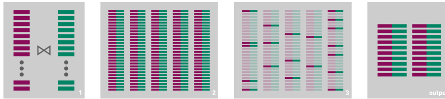
Figure 6.1: A depiction of executing a data frame query that joins two data frames and then filters the results. If the predicate is sufficiently selective, most of the output tuples will be discarded.
