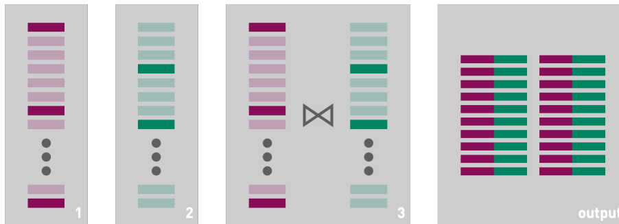
Figure 6.2: A depiction of executing a data frame query that filters two input relations before joining the results. If the predicate can be evaluated on each input relation independently, this query execution produces the same results as the query execution in the previous figure, but much more efficiently.
