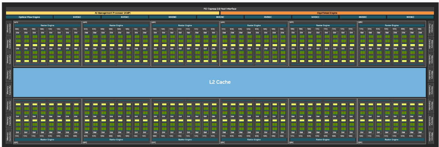
Figure 3. GB202 GPU block diagram (full chip).
