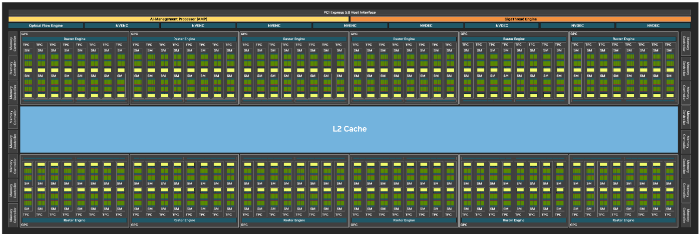
Figure 3. GB202 GPU block diagram (full chip).
