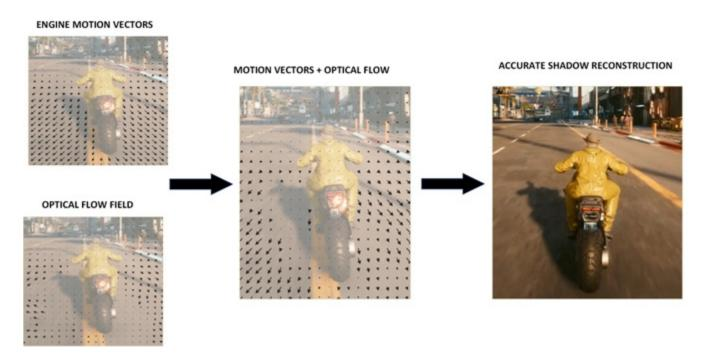
To generate more accurate frames without distracting artifacts, DLSS 3 combines game engine motion vectors with the OFA Engine's optical flow field.
