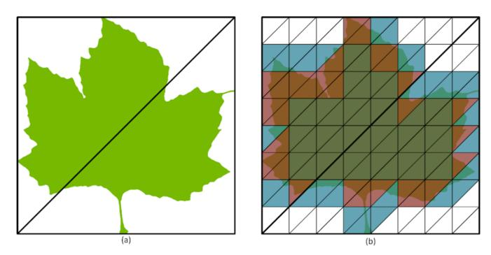
Opacity mask is applied to maple leaf which is composed of 2 triangles. The opacity engine evaluates the leaf and determines which sections are opaque, transparent, or unknown (in which case it must be sent back to the SM).
