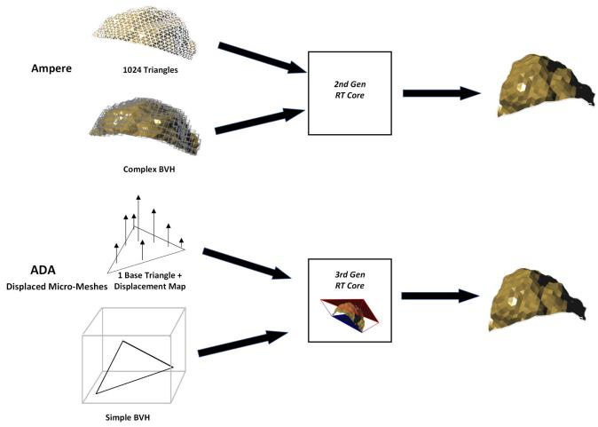
Ada's Third-Generation RT Core with Displaced Micro-Mesh Engine uses a simple BVH, 1 base triangle + displacement map to create a highly detailed geometric mesh with fewer required resources (both triangles and BVH structure) than Ampere's 2nd Generation RT Core.
