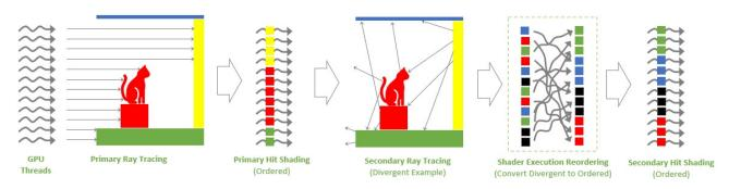
Shader Execution Reordering. Advanced lighting techniques such as path tracing cause shader divergence as secondary rays bounce off objects in the scene (denoted by various colors). In these scenarios, SER reorders shading work to improve efficiency.
