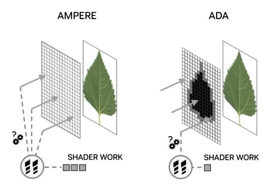
Ada's Opacity Micromap Engine with opacity mask reduces shader work compared to Ampere
