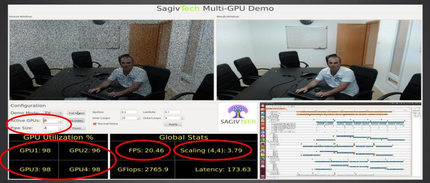
Four GPUs Four pipes Utilization: 96%+ FPS: 20.46 • Scaling: 3.79 – Near linear Scaling: Note NO gaps in the profilerGINTECH
