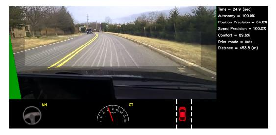
Figure 6: Screen shot of the simulator in interactive mode. See Section 7.1 for explanation of the performance metrics. The green area on the left is unknown because of the viewpoint transformation. The highlighted wide rectangle below the horizon is the area which is sent to the CNN.
