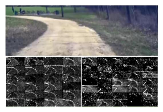
Figure 7: How the CNN "sees" an unpaved road. Top: subset of the camera image sent to the CNN. Bottom left: Activation of the first layer feature maps. Bottom right: Activation of the second layer feature maps. This demonstrates that the CNN learned to detect useful road features on its own, i. e., with only the human steering angle as training signal. We never explicitly trained it to detect the outlines of roads.
