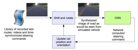
Figure 5: Block-diagram of the drive simulator.
