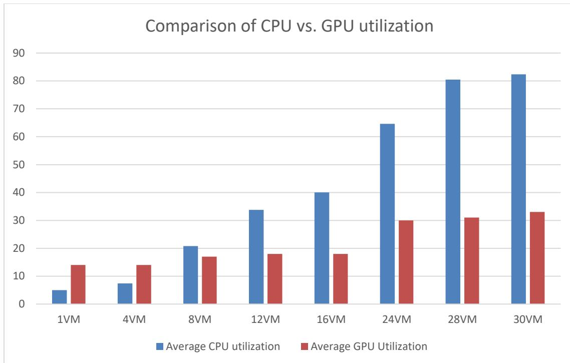
Figure 3 CPU and M60-1Q GPU Utilization
