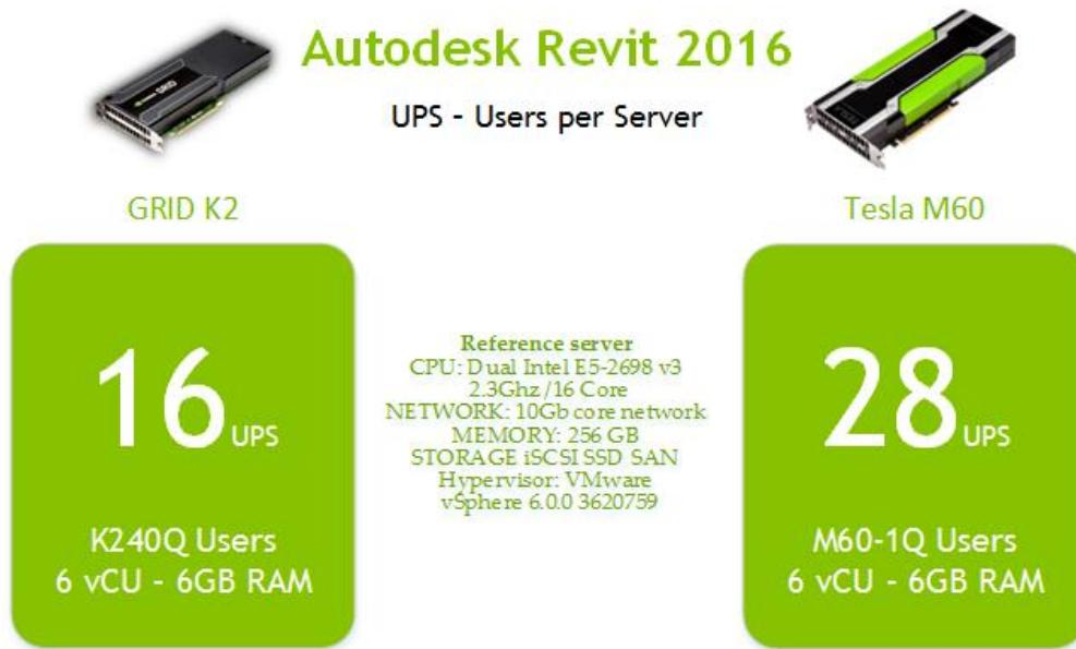
Figure 1 Autodesk Revit 2016 Users per Server for GRID K2 and Tesla M60
