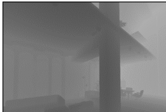
Rasterize depth buffer at headset eye positions
