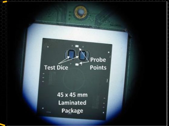
Test Chip #1 on Board
